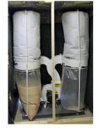
At left you can see my 3HP dust extractor in its soundproofed box. The bag on the left shows the strata of large shavings from a typical thicknessing session.
